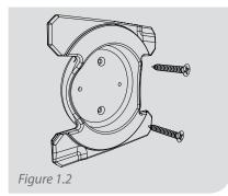
Use the wall bracket (P/N: 08-231) and appropriate screws to secure the wall mounting bracket to a suitable wall.
