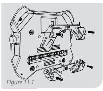
If the Mounting Brackets (P/N: 08-425) break, you can replace them by removing the two screws securing each bracket. Remove the broken bracket and replace with a new bracket. Secure the new bracket with the provided (UNC 10-24 x  $\frac{3}{4}$ ") screws.
