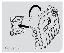
Position the monitor so that the green brackets on the back line up with the mounting bracket, turn clockwise until the monitor clicks into place.
