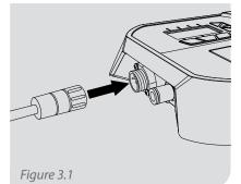
Connect the power supply by screwing it onto the receptacle on the left side of the unit (next to the air inlet fitting.) Plug the AC Adaptor into a power source.
