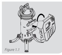
Position the monitor so that the green brackets on the back line up with the mounting bracket on the side of the RADEX<sup>®</sup>, turn clockwise until the monitor clicks into place.
