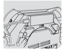
Tip: you can store the AC Adaptor between the tabs on top of the mounting bracket.
