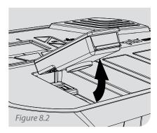
Lift the edge of the cartridge to remove it fully from the monitor. Replace with a new cartridge or a blank sensor cartridge.
