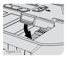
Each monitor comes with 3 blank cartridges. These should be placed into slots that are not currently being used to protect the electrical contacts and air supply manifold.
