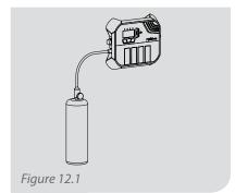
Connect the test air bottles to the air inlet.
