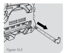
After removing the manifold, inspect it from all sides to make sure all of the holes are clear and that there is no oil or debris inside of the tube. DO NOT DISASSEMBLE THE MANIFOLD. If there is oil or debris inside of the manifold a replacement manifold (P/N: 08-422) must be used.
