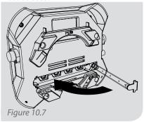
Rotate the manifold into the back of the monitor so the clip goes into the notches on the back of the monitor making sure it is securely clipped in.
