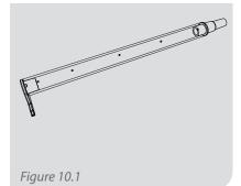
In the back of the GX4, there is a manifold (to distribute the air to the sensors) comprised of a clear tube with endcaps. This needs to be checked regularly to ensure it is clear of oil and debris. Note: Evidence of oil indicates an air supply issue that needs to be resolved.
