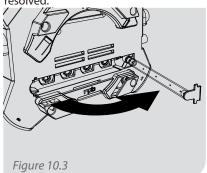
Rotate the manifold so it is sticking straight out from the back of the monitor.
