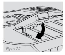
Insert the cartridge into any of the 4 slots in the monitor. First locate the top end so the tabs line up, then push the bottom until it clicks.
