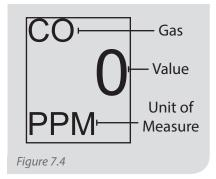
Each cartridge is represented by a box on the home screen. Each box shows the gas type, units of measure and the current reading.
