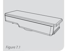
The gas detection sensors are supplied in individual cartridges. Select the cartridge for each gas you wish to detect at the correct alarm threshold for your region.
