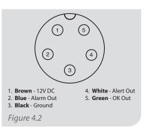
To configure your own external device, use the bare end AUX cable (08-434). It is recommended to use a qualified electrician when wiring to ensure you do not damage the electrodes.
