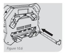
To replace the manifold, insert the tapered end into the green ring of the push-lock fitting inside the back of the monitor. Orient the holes in the manifold towards the sensors.
