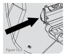
To remove the manifold for inspection, press in the green clip so it can be pulled out through the notches of the monitor case.
