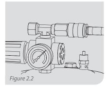
Connect the air supply hose to a Grade D air source regulated to between 7 to 80 PSI (50-550 kPa). Maximum air flow is achieved at 20 PSI.
