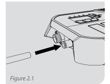
Insert the 3/8" O.D. Air Supply Hose (P/N: 08-428) into the push-lock fitting on the left side of the monitor. To disconnect, press the outside ring of the push-lock and pull the hose out. Note: Hose can be trimmed to the desired length.
