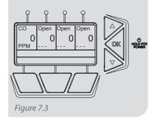
The cartridge will appear on the screen in the box that correlates to the slot it was placed in. The corresponding light above the screen will glow red or green to indicate the status.
